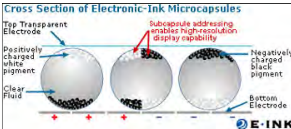
Figure 3. Principle of electronic paper, courtesy of E-ink Technology.
